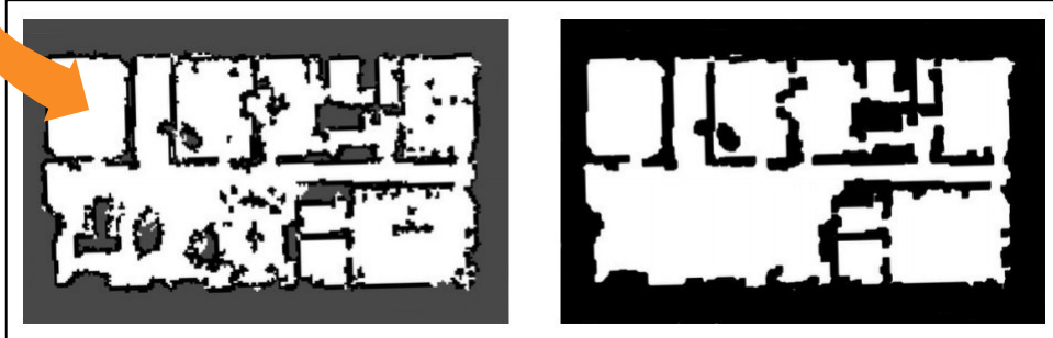
B Through the method of RoomSeg, you turn a cluttered occupancy grid into a nicely segmented map of the space.
