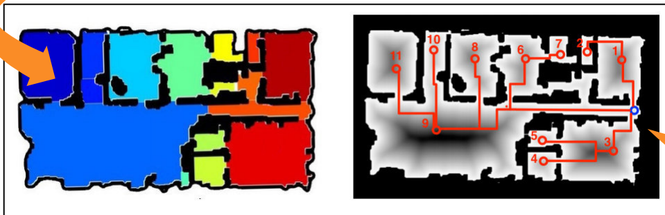
C Use the kind of CPU power to segment the occupancy grid into a bunch of different rooms to make it understandable for humans.
