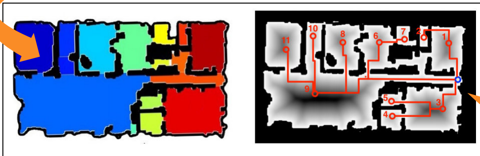
C Use the kind of CPU power to segment the occupancy grid into a bunch of different rooms to make it understandable for humans.
